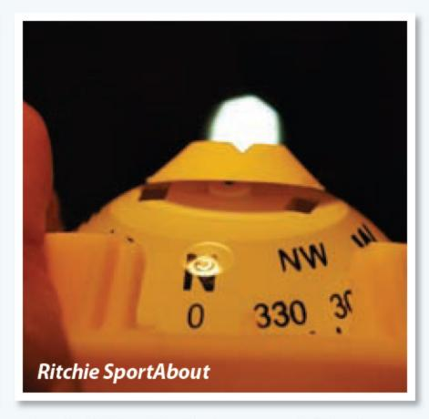
Is a lubber line helpful or hindering? That's largely a matter of taste. Our testers had difficulty lining up sighted objects using the Brunton Nexus and the Plastimo 100's lubber lines, but testers found the Ritchie SportAbout, which does not have a lubber line, to be equally difficult as it doesn't have an optical card reader.
