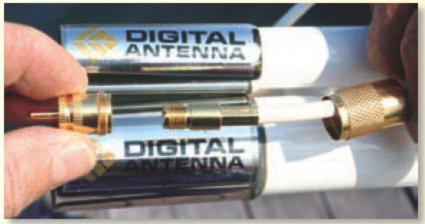
Clean connections at the coaxial terminals is essential to preventing loss of signal strength.
