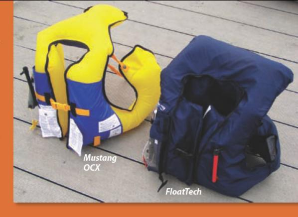
Testers fully inflated the bladders of the inflatable float coats and noted how long each held its air. The Mustang OCX bladder (left) lasted 11 hours, while the FloatTech (right) made it more than 20 hours despite the fact the ambient temperature fell about 15 degrees that night.
