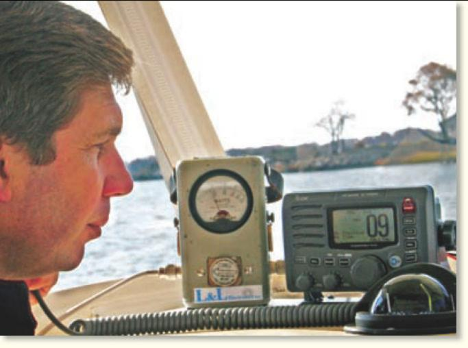
We used a Bird Model 43 wattmeter to measure the output of the ICOM 504 DSC VHF radios on our test boat.
