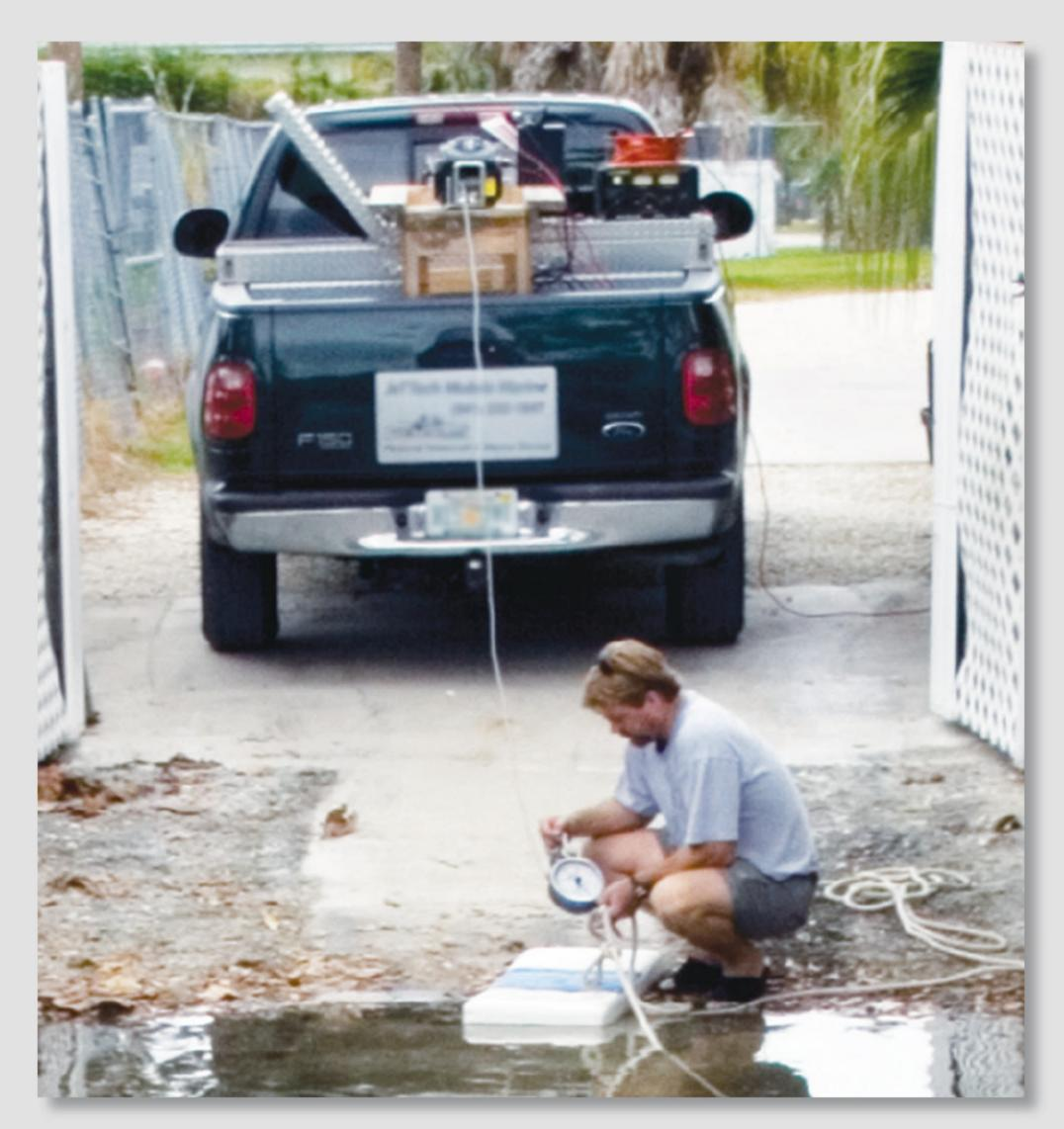
Testers carefully watched the Dillon dynamometer to note the pull pressure at which each anchor dragged.
