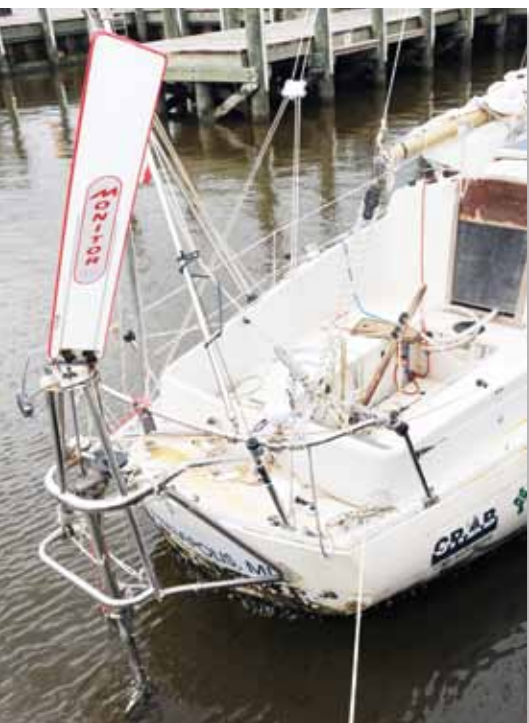
A tried and true stainless-steel Monitor windvane did most of the helming.
