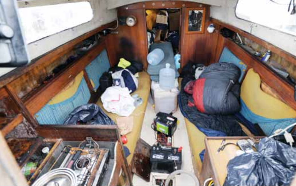
Rutherford's boat was in recovery mode in the days after his arrival in Maryland. Note the bolted reinforcement beam under the mast (above the V-berth doorway).
