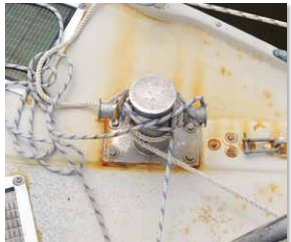
Rutherford set his sea anchor from a bitt that was through-bolted and linked by tie-rod to the stem.
