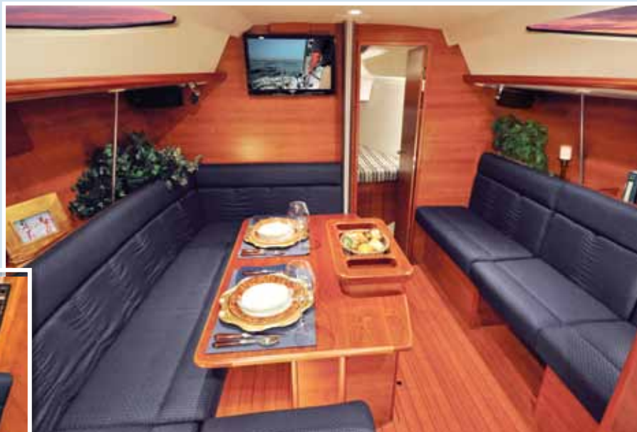
The main saloon table cranks down to convert to an 85-inch long berth (above). The 33 is the first of Hunter's new models with a Yanmar saildrive (above left). A middle section in the starboard settee (left) converts to small table.
