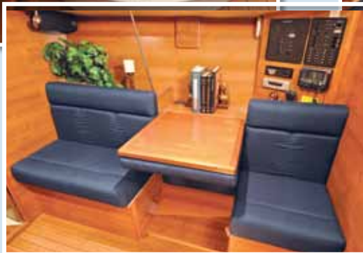
The main saloon table cranks down to convert to an 85-inch long berth (above). The 33 is the first of Hunter's new models with a Yanmar saildrive (above left). A middle section in the starboard settee (left) converts to small table.
