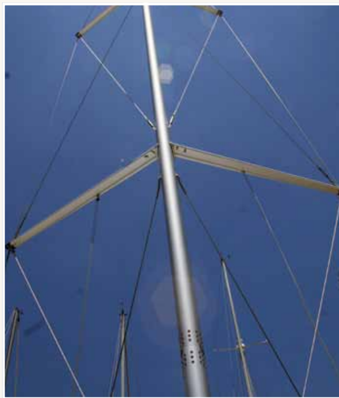
The Hunter 33 features the 15-degree swept-back spreaders that are the hallmark of the backstayless Bergstrom and Ridder (B&R) rig that Hunter favors.
