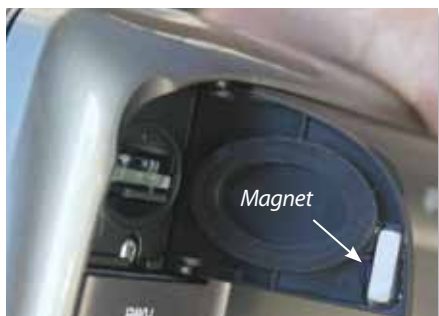
A close-up photo shows the magnet latch on the e7’s micro SD card slot.
