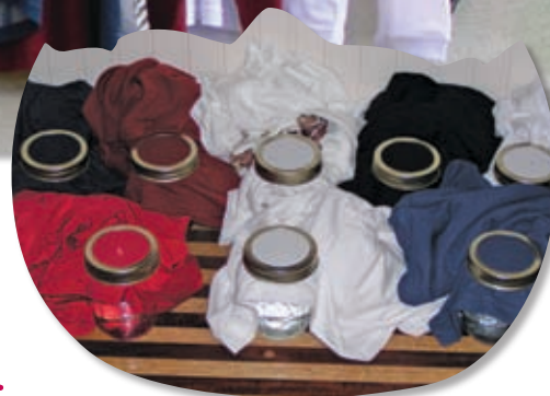
Right: In the evaporation test, we secured the shirts over jars of water and 'baked' them at 110 degrees for three hours.
