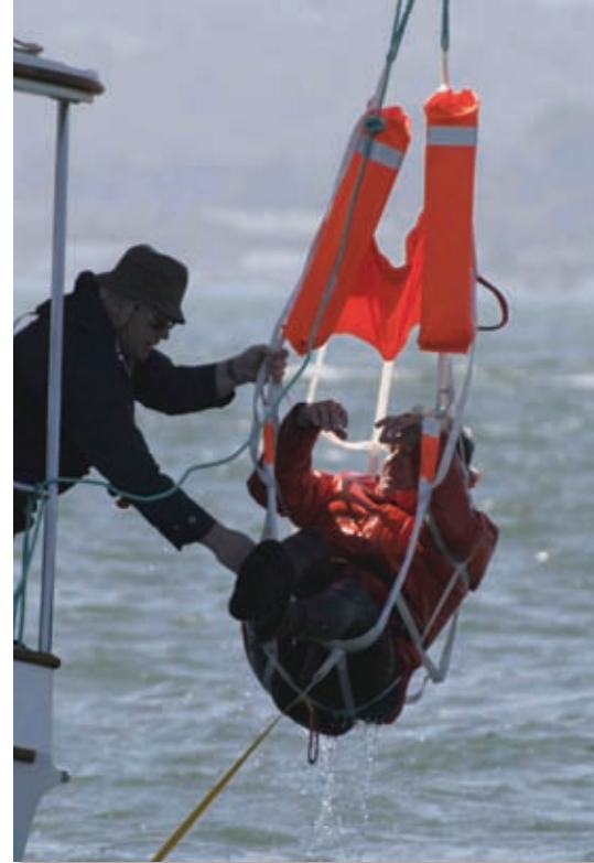
Top: A cradle of straps and lines, the Markusnet offers a secure ride for a helpless victim, but it is bulky, complicated, and difficult to climb into.
