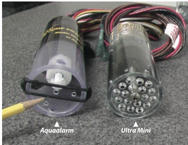
Left: We prefer the rugged Ultra Mini (on right) to the cheaper Aqualarm (with a pencil indicating the elastic retaining latch).
