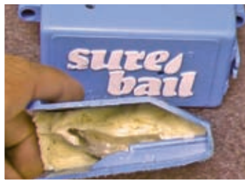
A cutaway view of the Sure Bail's float arm reveals its mercury capsule.
