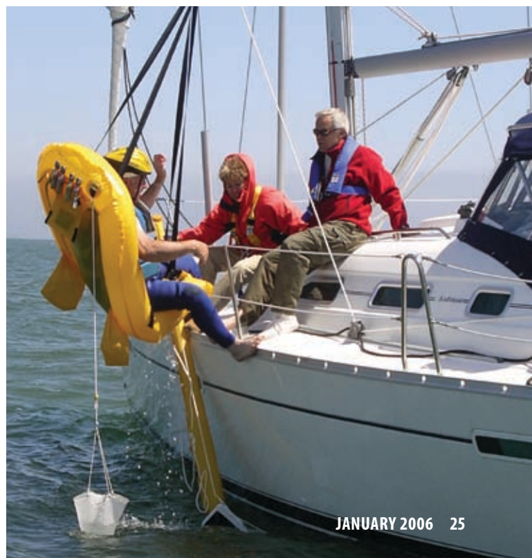
Bottom Right: The MOM9’s raft and sea anchor lack drains, so the ride is uneasy for the victim and hoisting the device is difficult.
