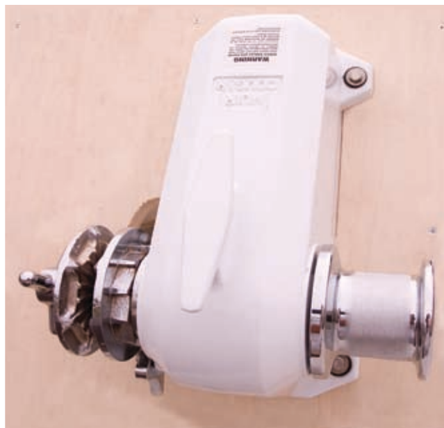
Left: With 300 watts of additional power the Lewmar H3 performed notably better than its sibling, the H2. Right: The Muir Cougar, right, comes standard with a capstan for handling nylon rode.
