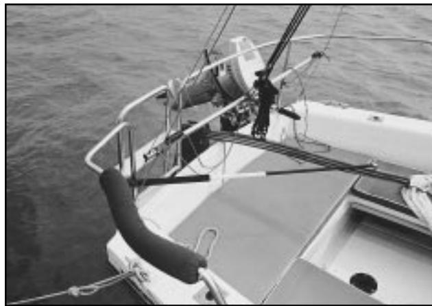
***Above left:** When raised, the pop-top gives 6' 4" headroom below. It is unusual in its use of telescoping supports. When it's down, headroom is about 50". Above right: The mainsheet traveler is a rod extended between the twin backstays—handy to the helmsman, and it cushions the effect of a jibe, but what about wear on the rig?*
